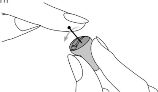
To switch the device off, open the battery compartment fully.
