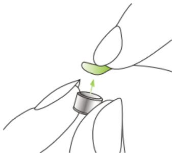
Open the battery door on the Roger Earpiece, and hold the earpiece so the door is on the right. Insert the battery into the door with the + symbol on the battery facing towards you.
