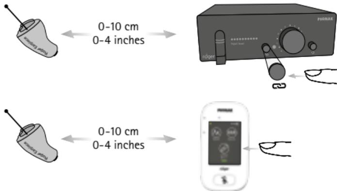
Only one Roger Earpiece can be connected at a time. Keep any other Roger devices out of range during this process. An unlimited number of Roger Earpieces can be connected.
